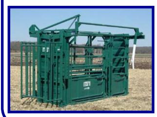
The Exotic Heavy Duty model caters for the top of the range buyer that expects their cattle handled by a crush that is second to none. This model has a lever operated parallel squeeze that can easily move a large animal to the centre of the crush with minimum effort. The animal operator is safely protected by a ratchet and pawl system that prevents the lever from moving. The Exotic Heavy Duty model caters for long and larger cattle.
